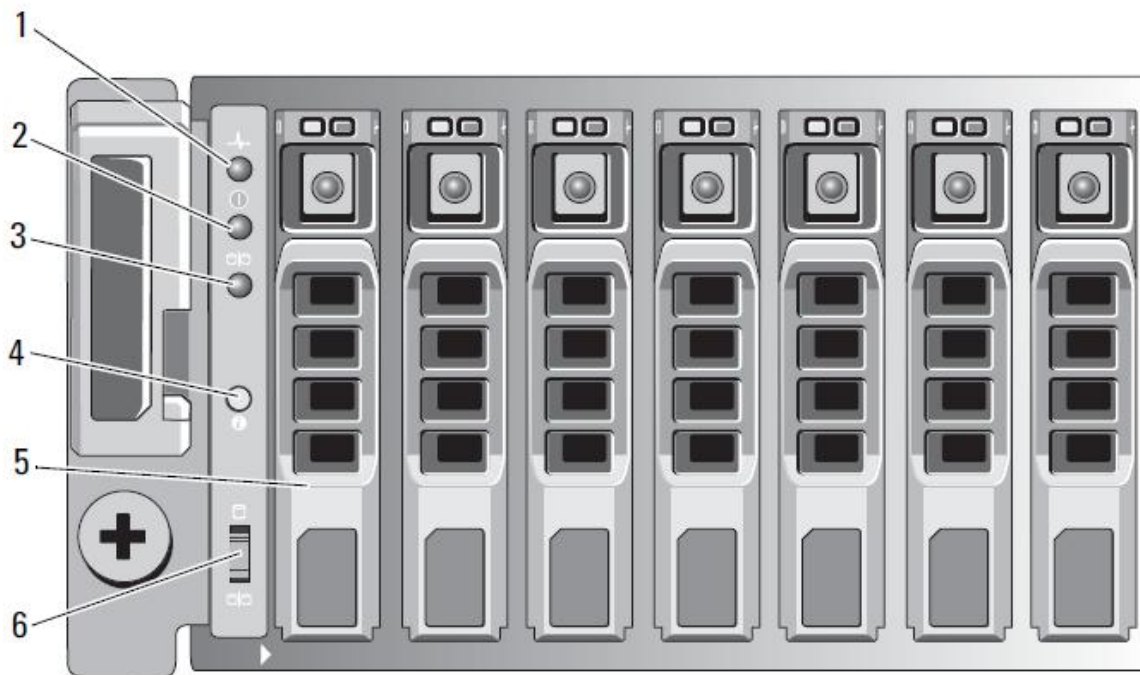
Figure 7. MD3200i Front Panel Indicators
